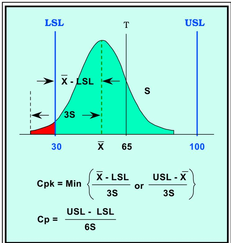
The Cpk index can never be greater than the Cp, only equal to it. This happens when the actual process average falls in the middle of the specification limits.
